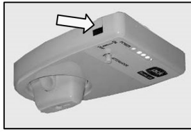
Enclosure base &amp; signal meter
