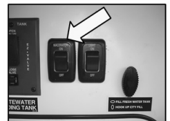
Macerator power switch
